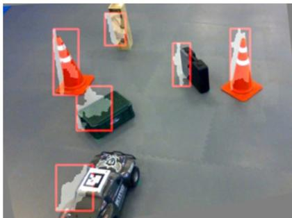
**Fig. 6** Detected obstacles by multi-UAV-based stereo vision system (baseline: 2132 mm)
