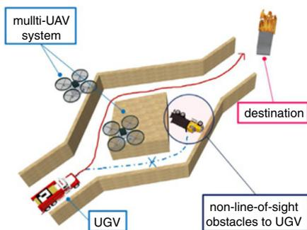
**Fig. 1** Operational concept of multi-UAV-based stereo vision system to assist UGV’s global path planning
