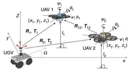
**Fig. 2** Coordinate frames of multi-UAV and UGV cooperative systems
