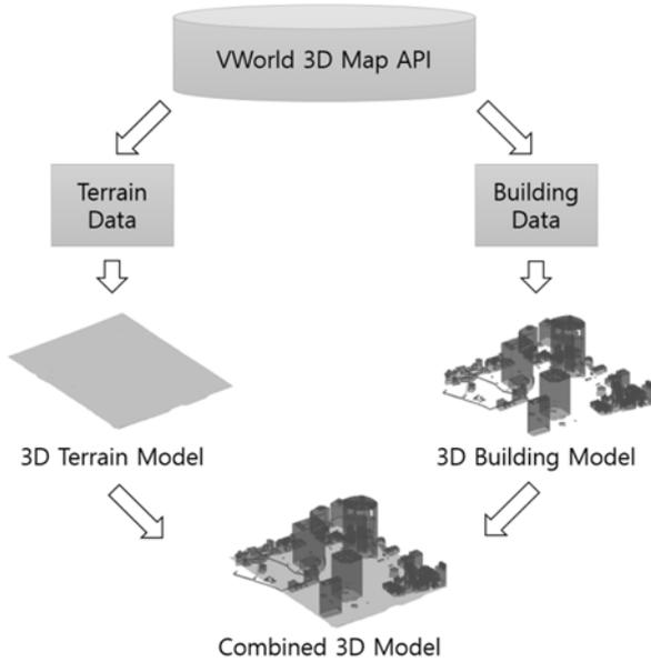
Fig. 1 Overall process for building the 3D model of a local area
