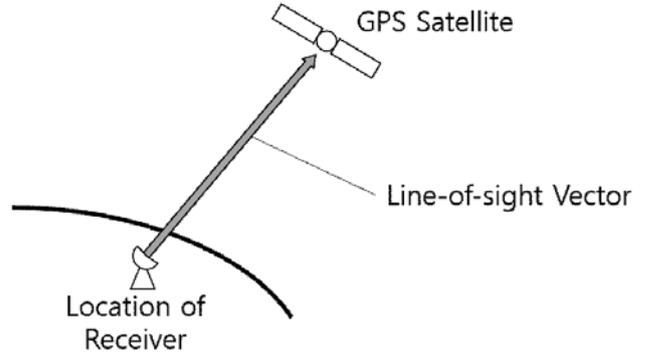
Fig. 2 Line-of-sight vector of a GPS satellite
