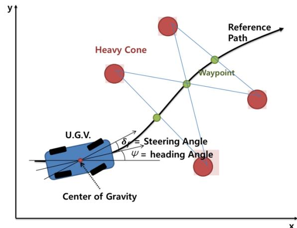
Figure 5. The implementation of steering control of UGV
