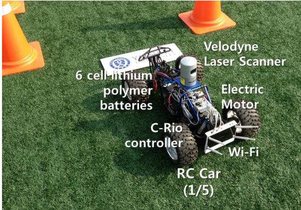
Figure 2. Components of UGV
