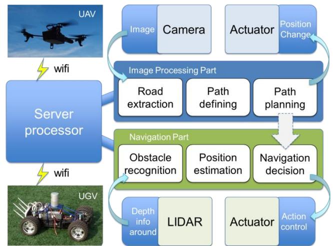
Figure 1. Architecture of the collaborative navigation system
