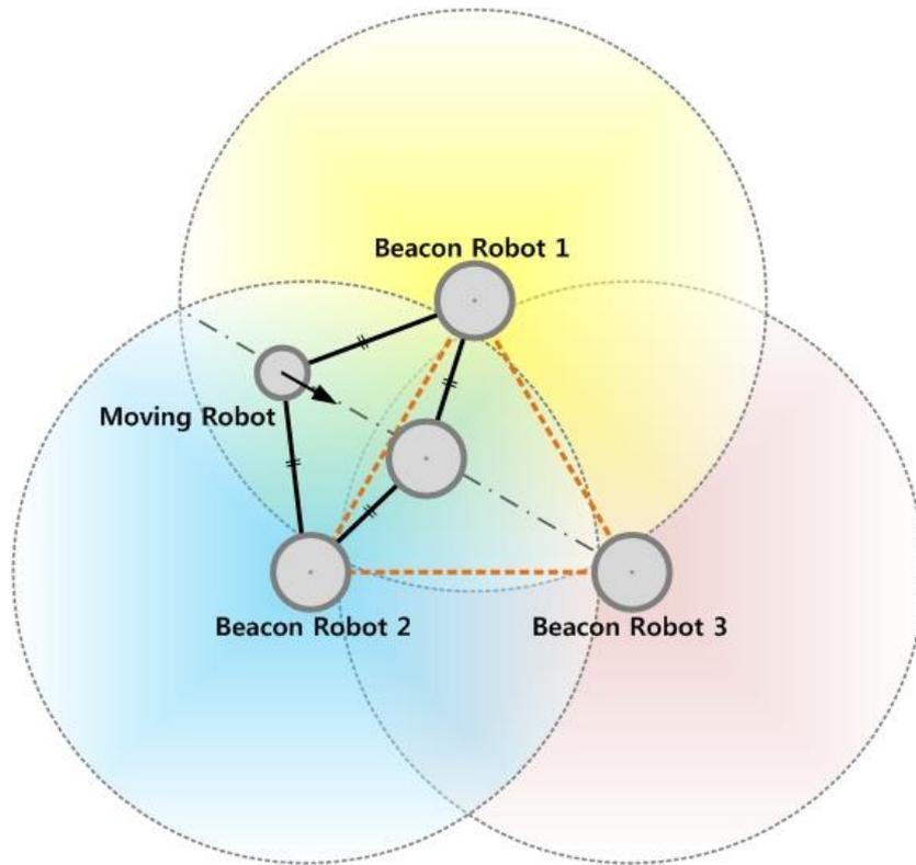
**Figure 4.** Localization of the moving robot using RSSI: operation of the moving robot that calculates the location using three RSSIs from the beacon robots.
