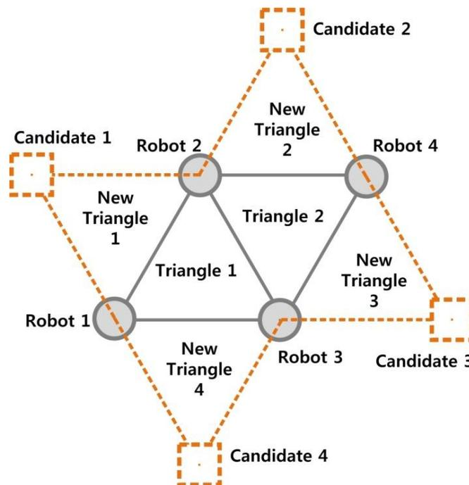
**Figure 2.** Formation with two connected triangles
