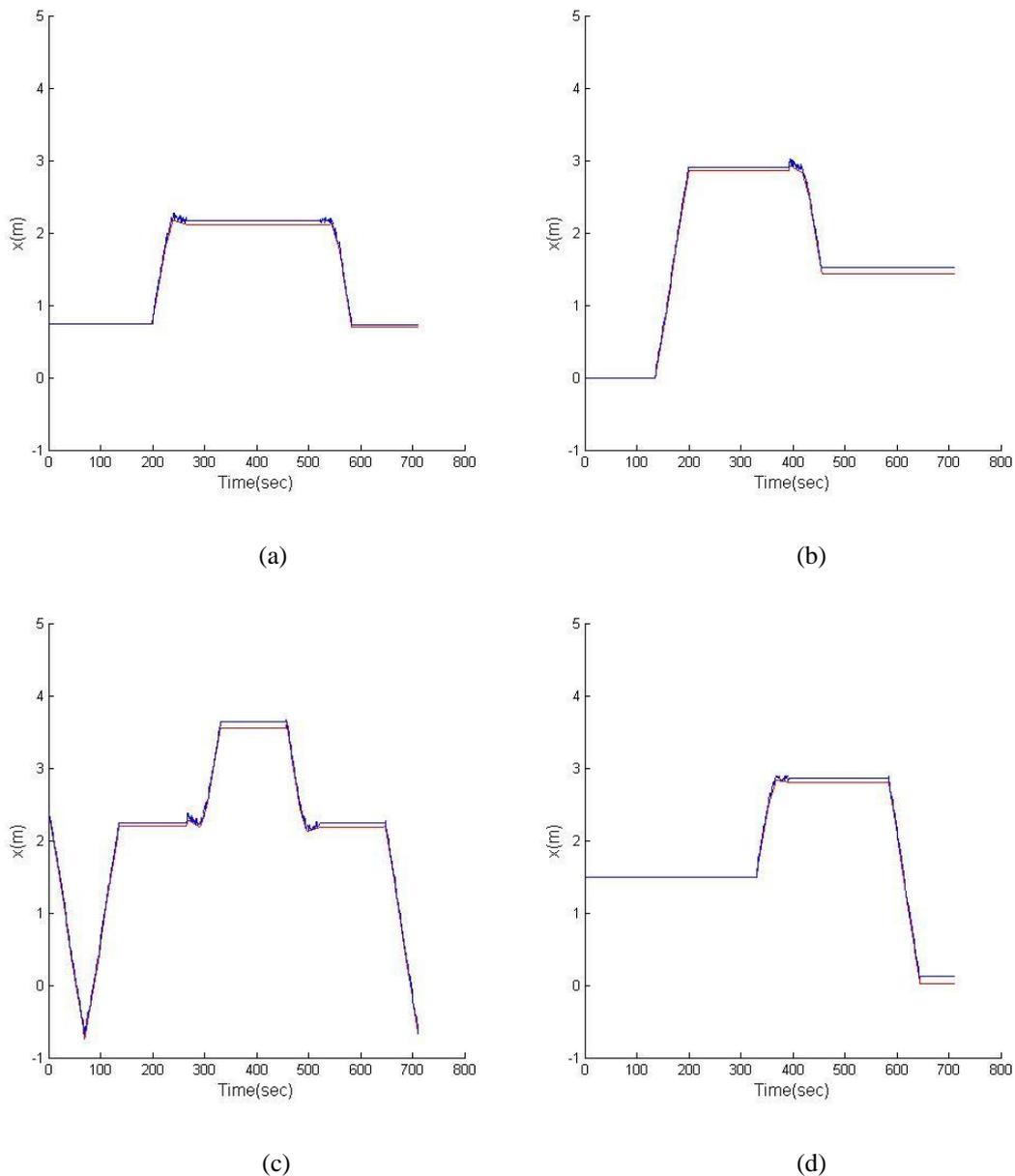
**Figure 8.** Ground truth position (red lines) and estimated position (blue lines) of the robots in the proposed triangular formation method: (a) position of robot 1 within x-coordinate, (b) position of robot 2 within x-coordinate, (c) position of robot 3 within x-coordinate, (d) position of robot 4 within x-coordinate.
