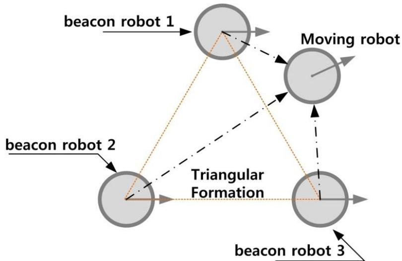
**Figure 1.** Localization system based on the triangular formation (orange dash lines: triangular formation and dash-dot arrow: calculated position by acquired distance information).
