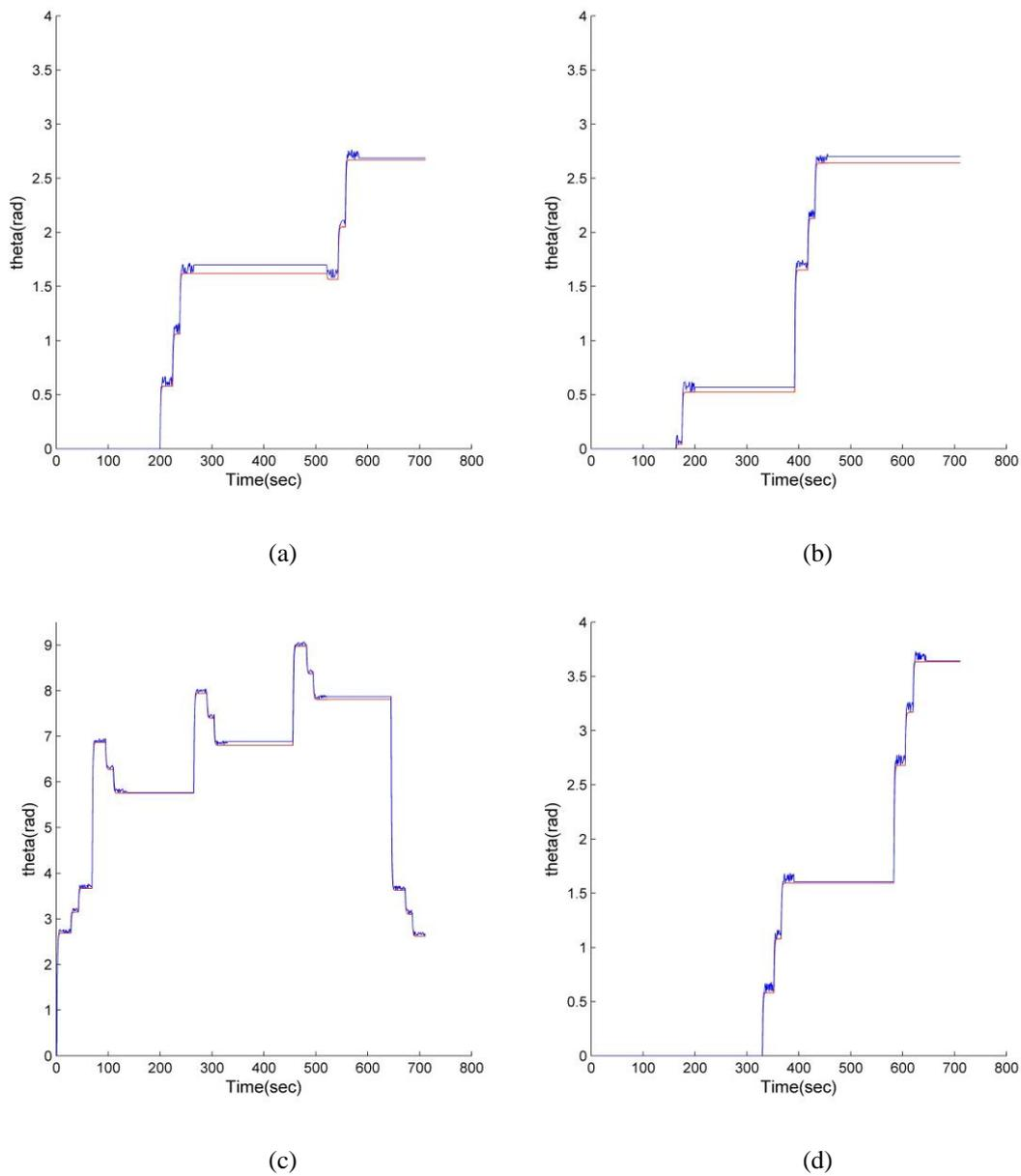
**Figure 10.** Ground truth position (red lines) and estimated position (blue lines) of the robots in the proposed triangular formation method: **(a)** heading angle of robot 1, **(b)** heading angle of robot 2, **(c)** heading angle of robot 3, **(d)** heading angle of robot 4
