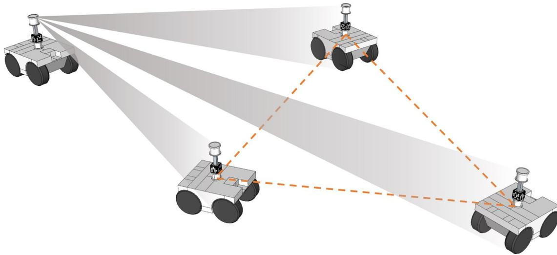
**Figure 5.** The artificial marker-based localization system
