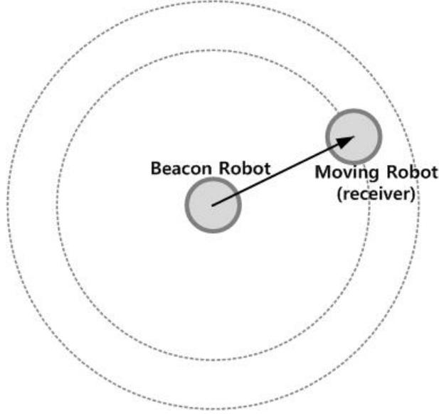
**Figure 3.** Localization of the moving robot using RSSI: Signal propagation from the beacon robot to the moving robot.
