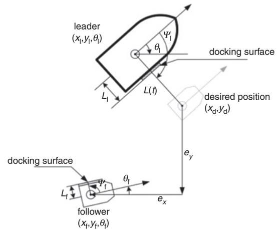
Fig. 1 Proposed docking formation with respect to docking surface
