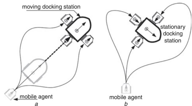
Fig. 2 Possible docking motions of agent according to mobility of docking station
