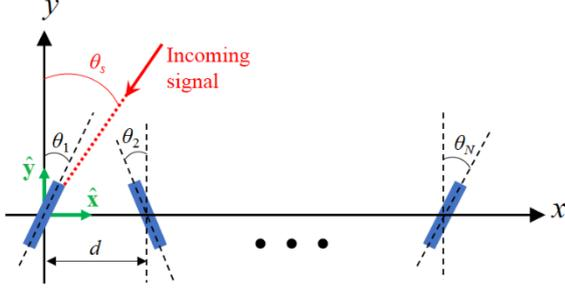
Fig. 1. A uniform linear dipole array with orientation misalignments.
