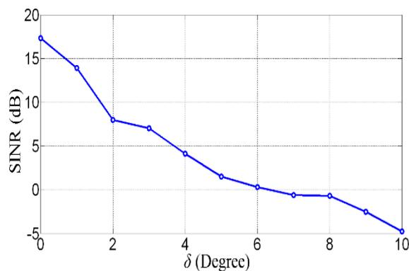
Fig. 2. SINR performance deterioration of the MVDR beamformer due to orientation misalignment.
