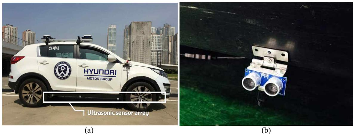
Fig. 1. (a) Hardware platform installed on the test vehicle, and (b) the implemented single ultrasonic sensor.
