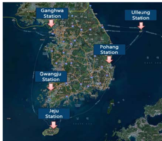
Figure 2 Initial plan of the transmitters locations of the future Korean eLoran system ([4], Figure 3 of [3])
