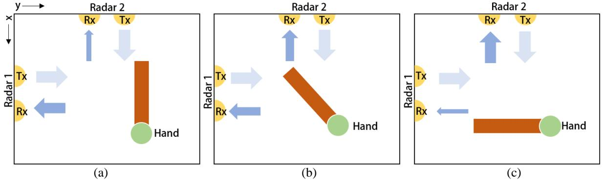
Figure 2. The relation between the power of reflected signals and user's hand posture in 2D space. (a) The case when the hand direction is parallel to Radar 1 (0 degree). (b) The case when the hand direction is slanted to both radars (45 degree). (c) The case when the hand direction is almost parallel to Radar 2 (90 degree).
