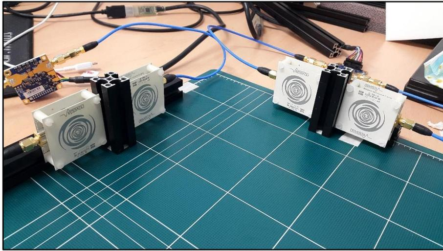
Figure.3. Test-bed for hand posture estimation method using multiple IR-UWB radars.
