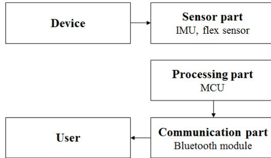
**Figure 1. Configuration of the mobile spinal curve detection device**
