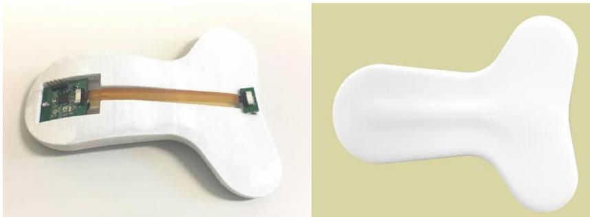
**Figure 3. The design of the mobile posture tracking device**
